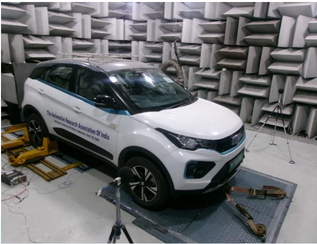
Figure 1: Vehicle with AVAS unit under test on Chassis Dynamometer
