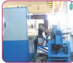
50KW Induction Billet Heater
