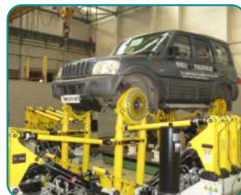
Full Vehicle level - 6 DOF Multi axis & 4/6 Post test set up
