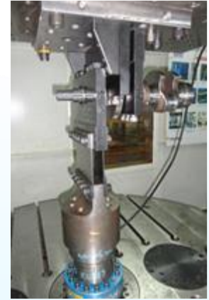
Fig 5: Crankshaft Fatigue Testing
