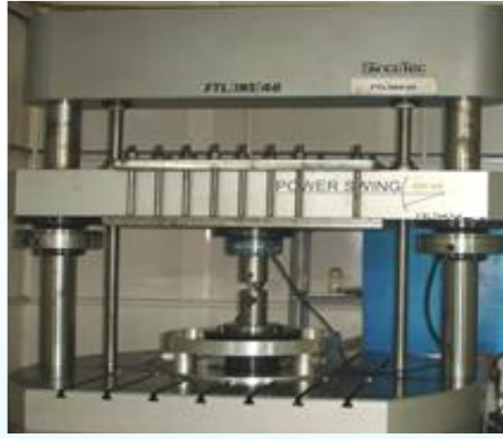
Fig 4: Connecting Rod Fatigue Testing
