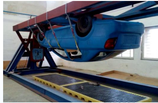
Static Rollover Facility
