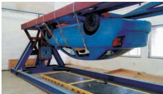
Static Rollover Facility
