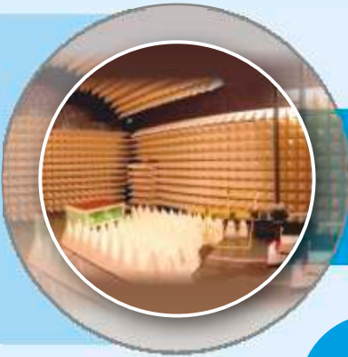
EMC Chamber for 2W, 3W, Automotive and Industrial Components
