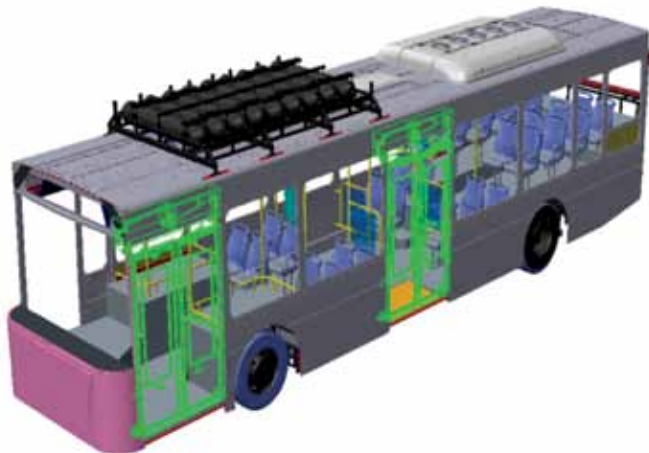
Figure 2 : Aluminium Bus Super Structure for City Bus
