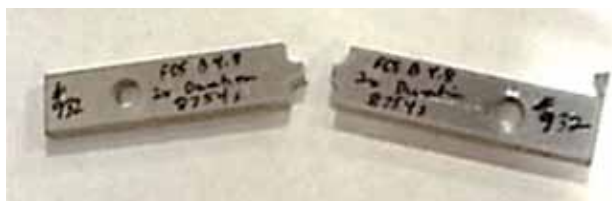
Figure 4 : Beam Fracture due to Fatigue
