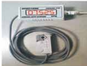
GASOLINE ENGINE RPM SENSOR WITH DISPLAY
