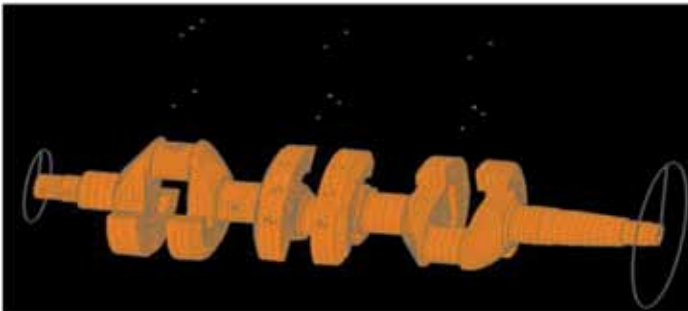
Figure 7 : 3D Crank Shaft Model Integrated with 1D Model in ENGDYN
