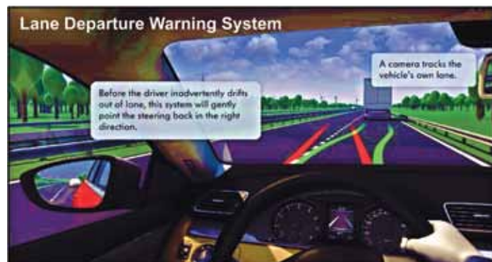
Figure 1 : Lane Departure Warning System
