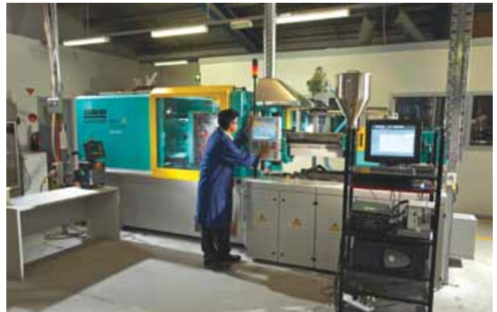
Figure 2 : Autodesk Moldflow Material Testing Lab. Best Practice Requires that the Inputs and Outputs from an Injection Molding Simulation Agree as Closely as Possible to the Actual Conditions of a Real-life Molding Machine.
