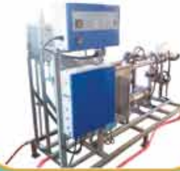
Hot coolant conditioning system
