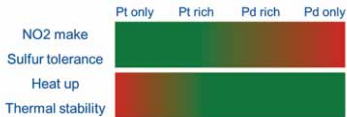
Figure 3 : Influence of the Pt/Pd Ratio on the DOC and CDPF Features
