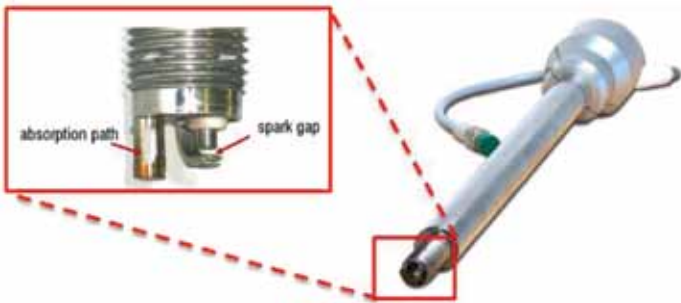
Figure 9 : ICOS System and M12 Spark Plug Probe
