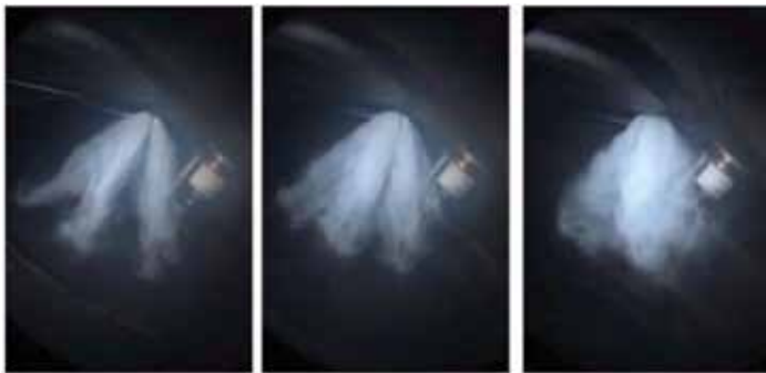
Figure 2 : Spray Pattern at Varying in-cylinder Pressure
