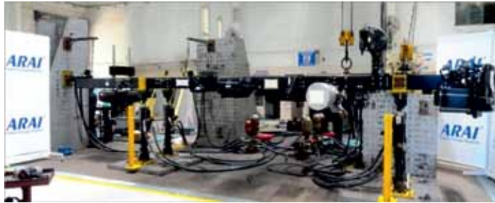
Figure 3 : Chassis Mounted on Actual Test Rig
