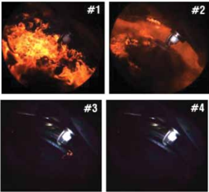
Figure 8 : First Four Cycles of a Cold Start with Visible Pool Fire from Piston and Wall Wetting
