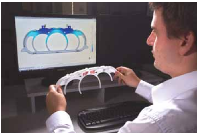
Figure 1 : Comparing Physical Testing with Digital Simulation. An Important Reason for Benchmarking is to Confirm Simulation Results When Users are First Introduced to Injection Molding Simulation Applications.
