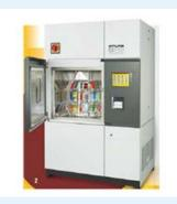
Radiation emitted by Xenon source are closest to solar radiations.
