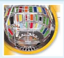
Radiation emitted by Xenon source are closest to solar radiations.
