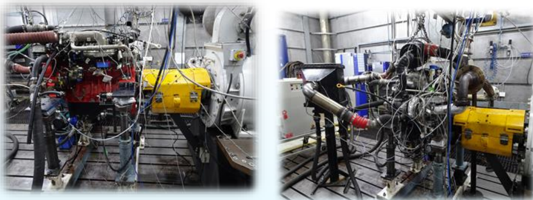
Test Engine set up on Engine Dynamometer for FFT Developmental Trial
